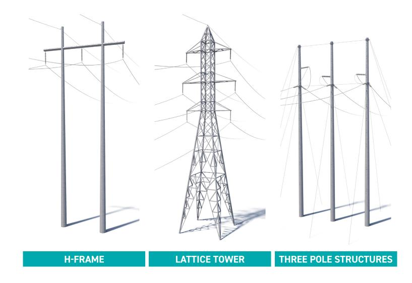
Crews plan to build the transmission line using a combination of structures such as steel H-frame poles, lattice towers and three-pole structures.
